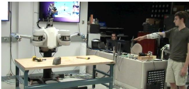
Fig. 4. Point-to-goal command to the manipulation robot: The user points to the impact driver of the left part of the table.
